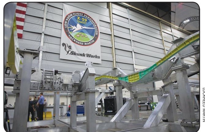
First spars in the jig emphasize the pronounced gulling of the inboard wing for low boom.
