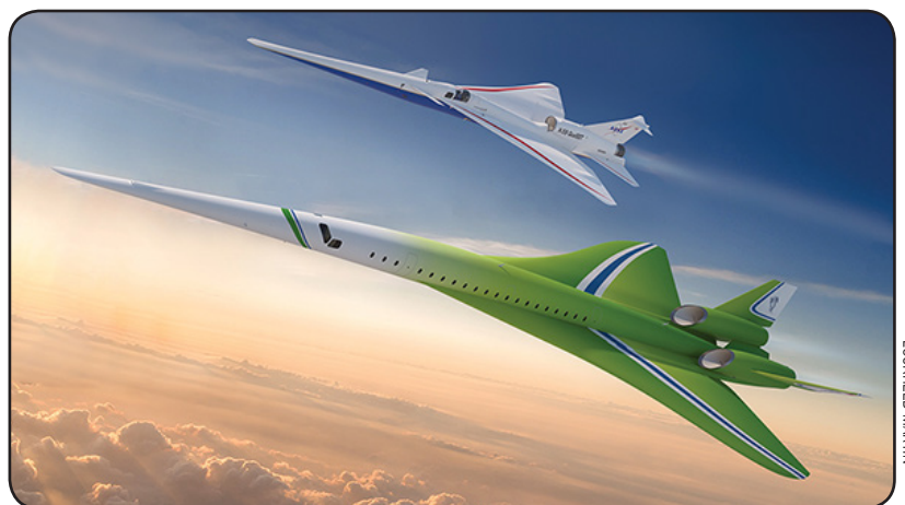
Lockheed Martin's 40-passenger quiet SST concept (foreground) draws on NASA's X-59 low-boom demonstrator (background).
